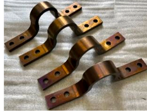
Fig. 7. Specimen of SMA-Ω damper.
